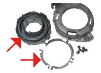
Fig. 4: Mechanical damage and overheating on the releaser
