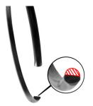
Fig. 3: Worn retaining ring. Consequence: Releaser will separate from the diaphragm spring → sudden clutch engagement
