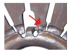
Fig. 5: Excessive wear on releaser ring and diaphragm spring fingers
